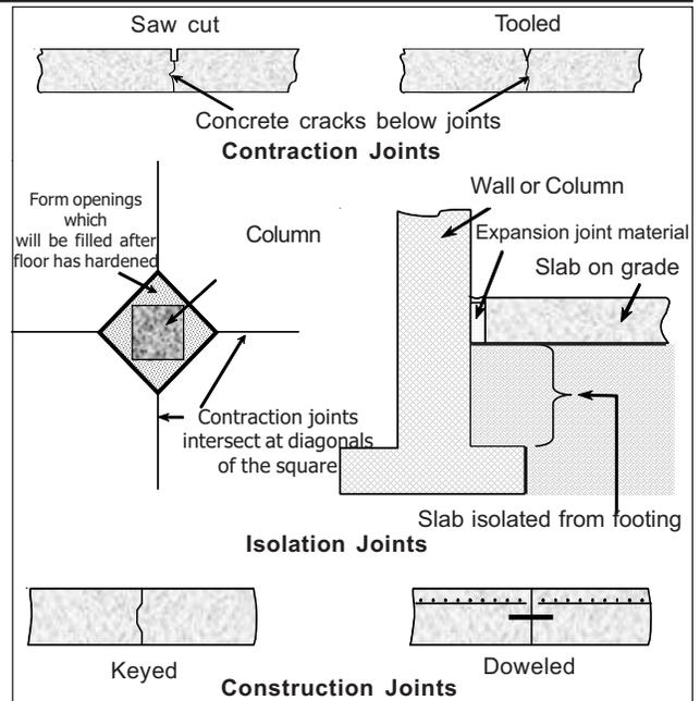
natural tendency to shrink is restrained, tensile stresses that exceed its tensile strength can develop, resulting in cracking.
